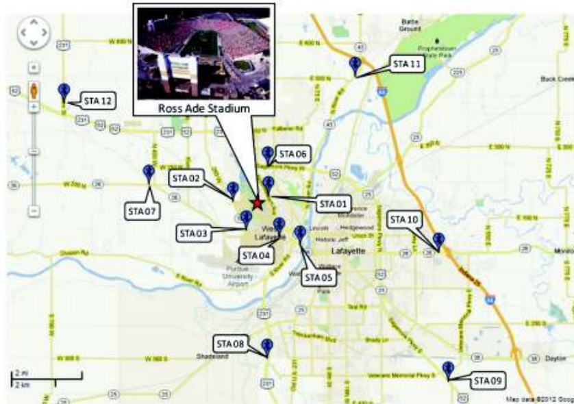
FIGURE 3. LOCATIONS OF BLUETOOTH MONITORING STATIONS SURROUNDING THE FOOTBALL STADIUM (DAY, ET AL., 2012)
